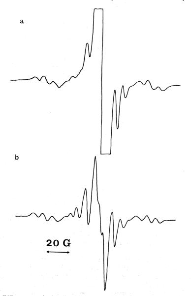
Fig. 1. – ESR spectra of  $\gamma$ -irradiated o-TSA; a) at room temperature before annealing b) at room temperature after annealing for a few hours at 48 °C. Magnetic field normal to the b axis, at 0° from the c\* axis. Power level approximately 20 mW.
