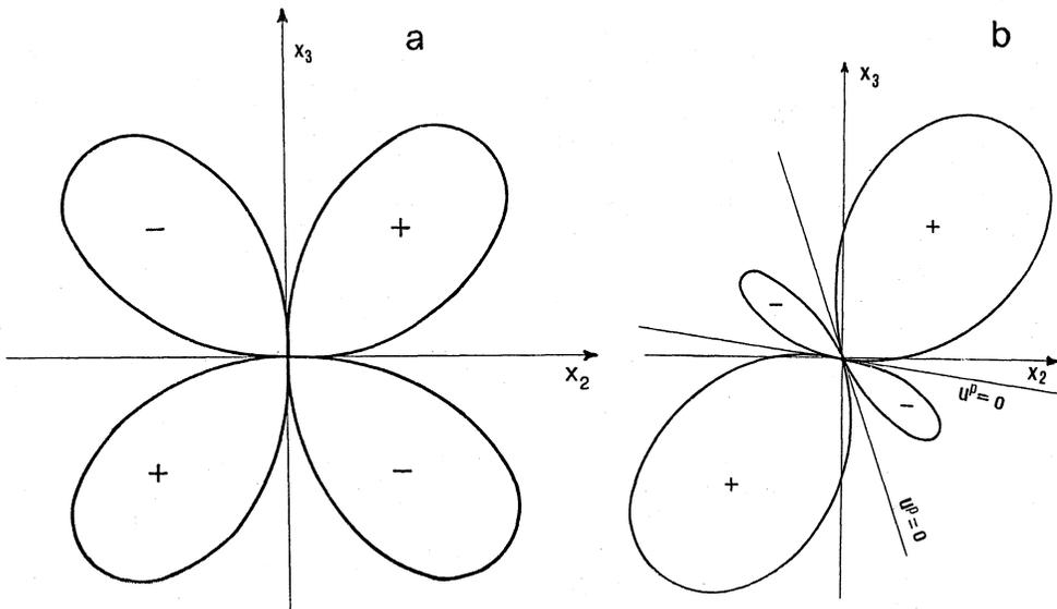
Fig. 2. - Radiation pattern for (a) a pure shear source and for (b) a source with a component of dislocation normal to the fault plane ( $u_3 = 0.2 u_1$ ).
