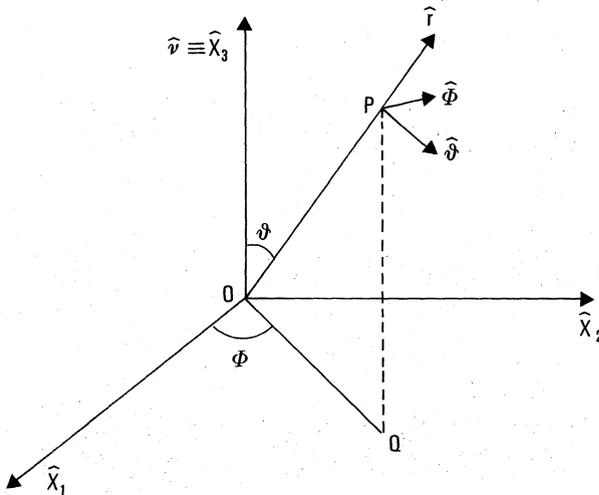
Fig. 1. - Coordinate systems used to determine the radiation patt.
