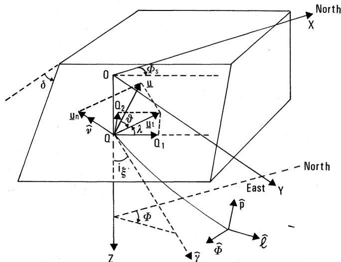
Fig. 4. — Coordinate systems and components of the displacement vectors used to solve the direct problem.
