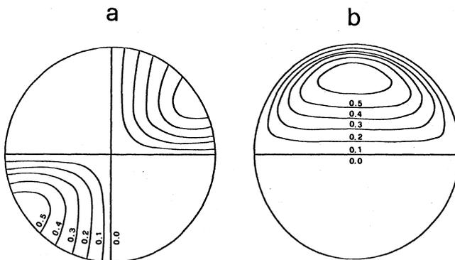
Fig. 3. - Nodal lines in the lower hemisphere projection for (a) a dip slip fault and for (b) a strike slip fault, shown for different values of the dislocation component normal to the fault plane.
