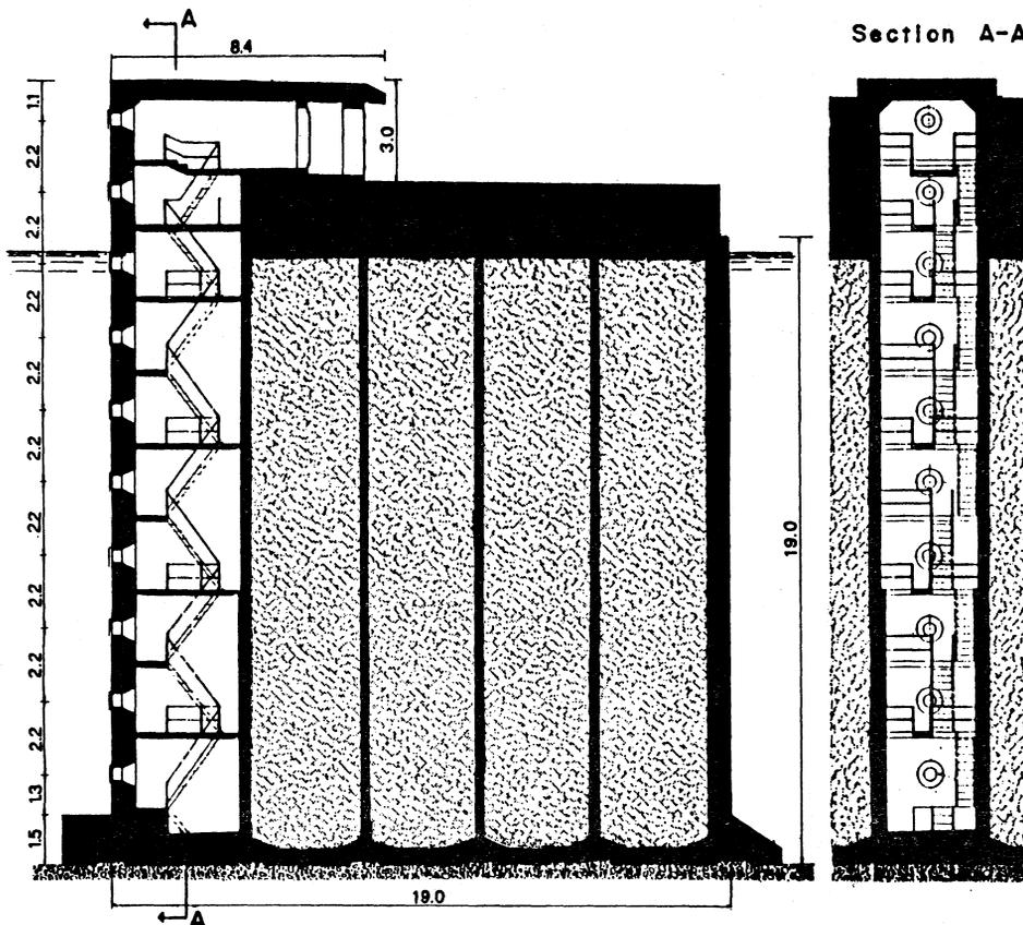
Fig. 1. - Station for measuring wave pressure against Genoa breakwater. The caisson is based on a rubble mound. Depth of the caisson base is nearly 17 m, depth of natural bottom is 25 m.
