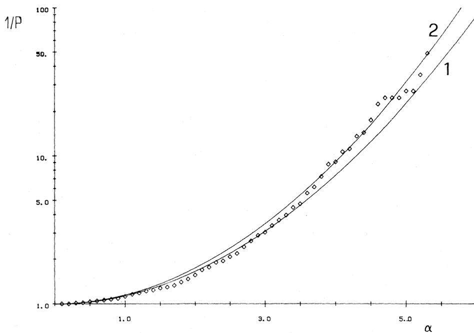
Fig. 6. - Swells: probability  $P(\alpha)$  that a wave taken at random is greater than  $\alpha \sqrt{m_0}$ . Line 1 represents eq. (7) and line 2 eq. (5) with  $a = -0.81$ .
