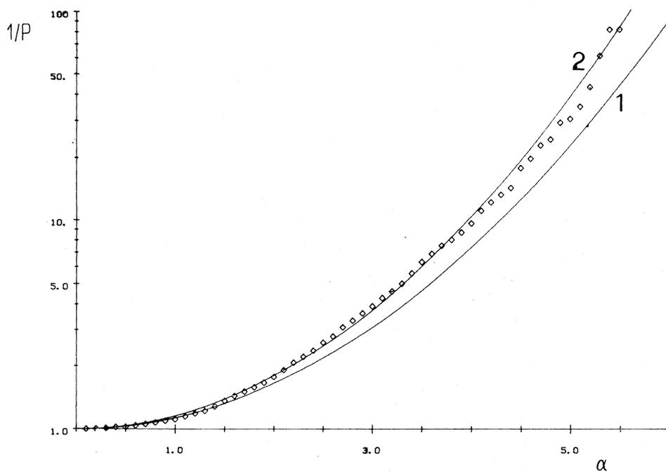
Fig. 5. - Storm seas: probability  $P(\alpha)$  that a wave taken at random is greater than  $\alpha \sqrt{m_0}$ . Line 1 represents eq. (7) and line 2 eq. (5) with  $a = -0.7$ .
