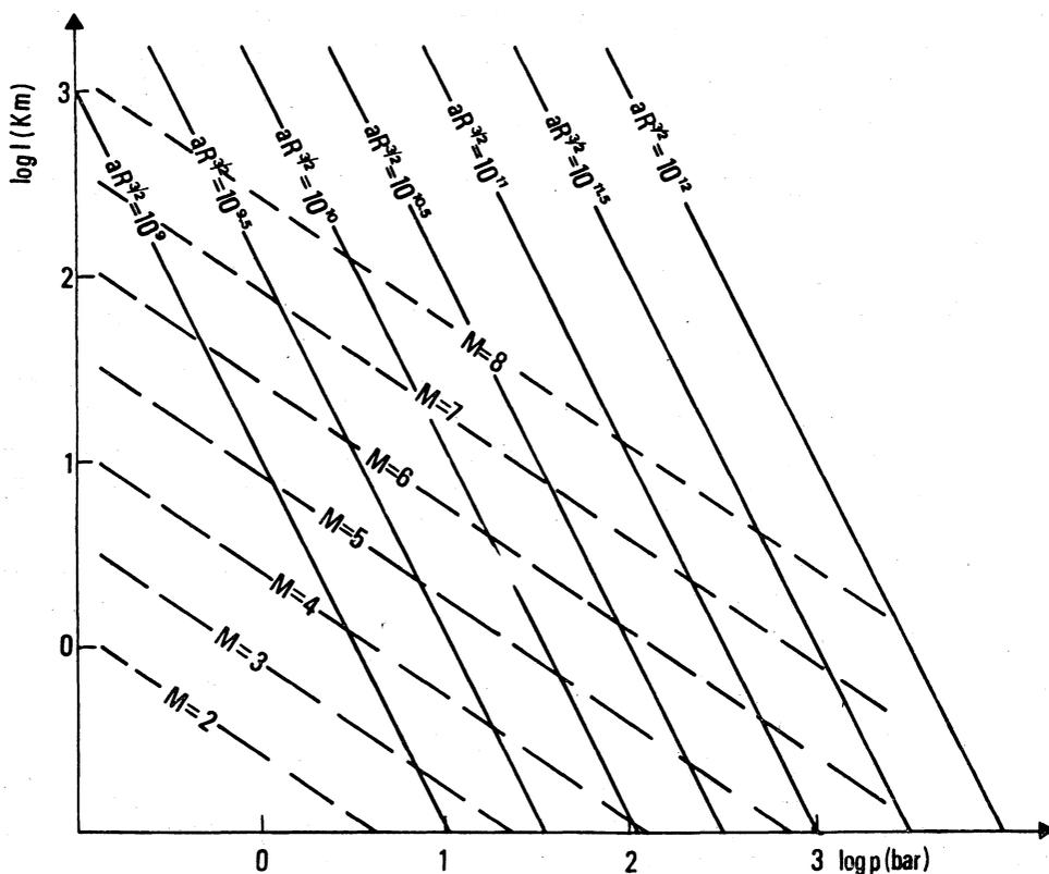
Fig. 2. - Isolines of magnitude and *rms* acceleration *a* in the plane of the linear dimension of faults *l* and stress drops *p*.
