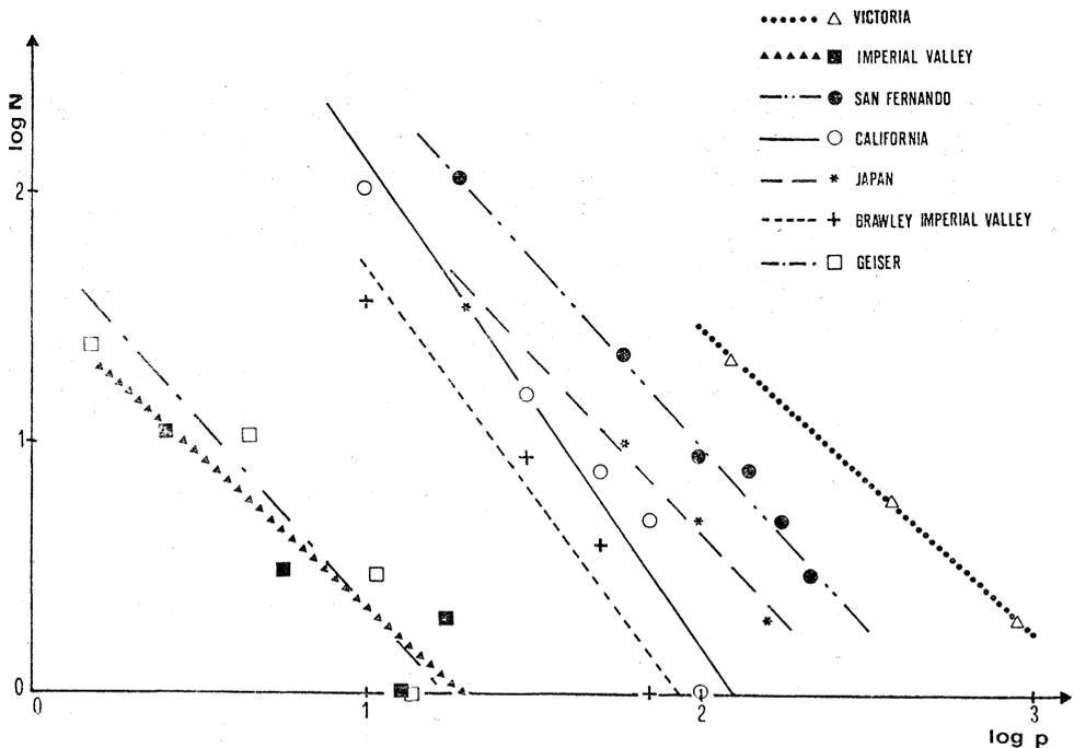
Fig. 1. - Linear regression for the stress drops of the 1971 San Fernando earthquake aftershocks (Tucker and Brune, 1973), of Japan (Mikumo, 1979; Utsu, 1979), of the Brawley-Imperial Valley, 1975 swarm (Hartzell and Brune, 1977), of Southern California (Thatcher and Hanks, 1973), of the Imperial Valley, 1977 swarm (Adair *et al.*, 1977), of scattered earthquakes in the Geiser (California) region (Peppin and Bufe, 1980) and of the 1978 Victoria (Mexico) swarm (Munguia *et al.*, 1978).
