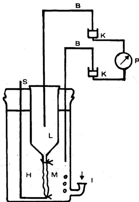
Fig. 1. - Experimental apparatus. M: midgut; L: lumen side chamber; H: hemolymph side chamber; P: Voltmeter; I: gas inlet; S: midgut support; K: Kalomel electrodes; B: agar-KCl bridges.
