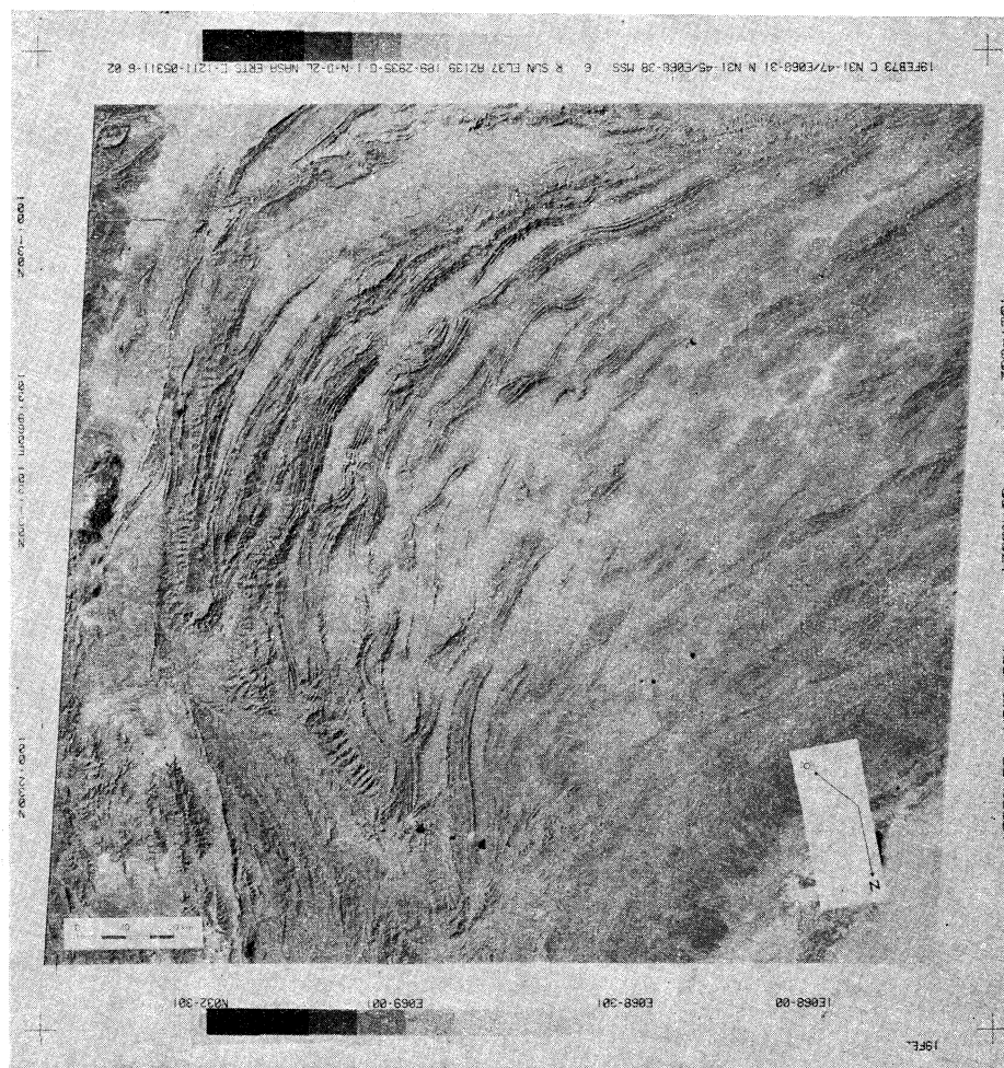
Fig. 6. - ERTS image of an area about 32^{\circ} N and 68.5^{\circ} E which was not used in the present work but shows how clear lineations can appear in an area of alternated erosion and sedimentation.
