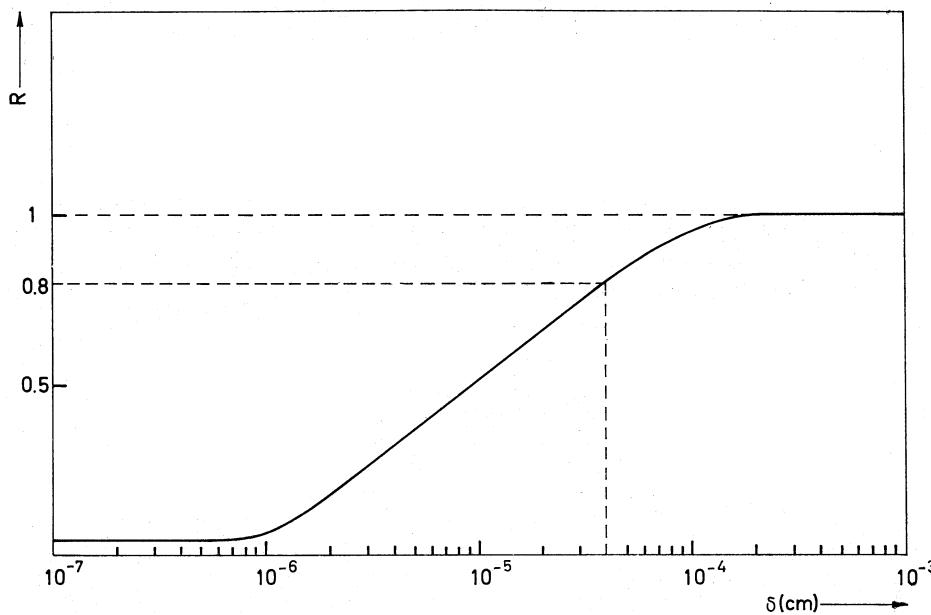
Fig. 1. - Ratio  $R = \left(\frac{dW}{dl}\right)_d / \left[2\left(\frac{dW}{dl}\right)_e\right]$  against the separation  $\delta$  of the  $e^+ e^-$  pair.
