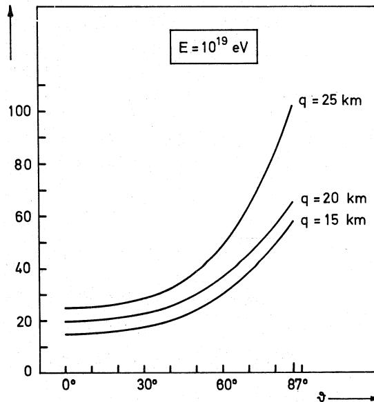
Fig. 3. - Distance travelled by the  $e^+e^-$  emitting as dipole against the angle of inclination to the vertical for 3 values of production quote (primary energy  $E=10^{19}$  eV).
