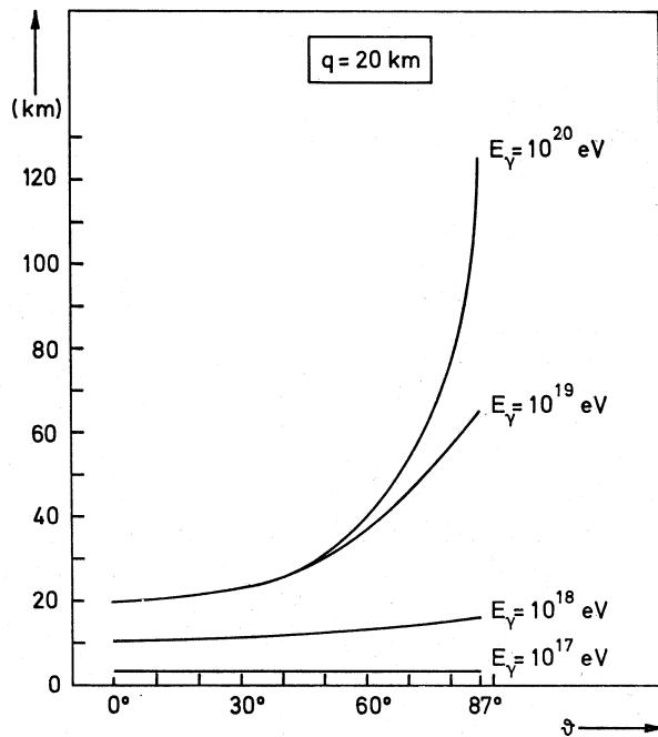
Fig. 4. – Distance travelled by the  $e^+ e^-$  pair emitting as dipole against the angle of inclination to the vertical for 4 values of primary energy (production quote  $q = 20$  km).
