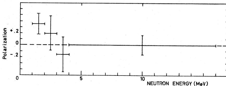
Fig. 2. - Polarization of photoneutrons from  ${}^7\text{Li}$ .
