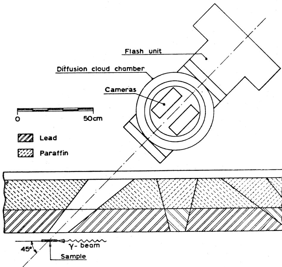
Fig. 1. - Diagram of the experimental arrangement.
